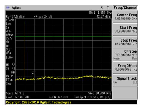
900 MHz, FSK High Channel (channel 82)
