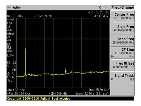
2.4 GHz, GFSK Low Channel (Channel 0), Gain Setting of 14
