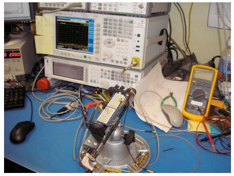
ANTENNA PORT CONDUCTED TESTS, CCS
