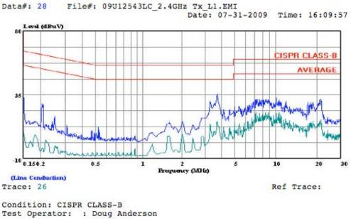
Test Operator: : Doug Anderson Project #: : 09J12543 Company: : Silver Springs Network EUT Description:: Power Meter Radio Module Mode: : 900MHz Tx Mode Target: : FCC Class B Voltage: : 115VAC/60Hz : L2: Peak ( Blue ) , Average (Green )
