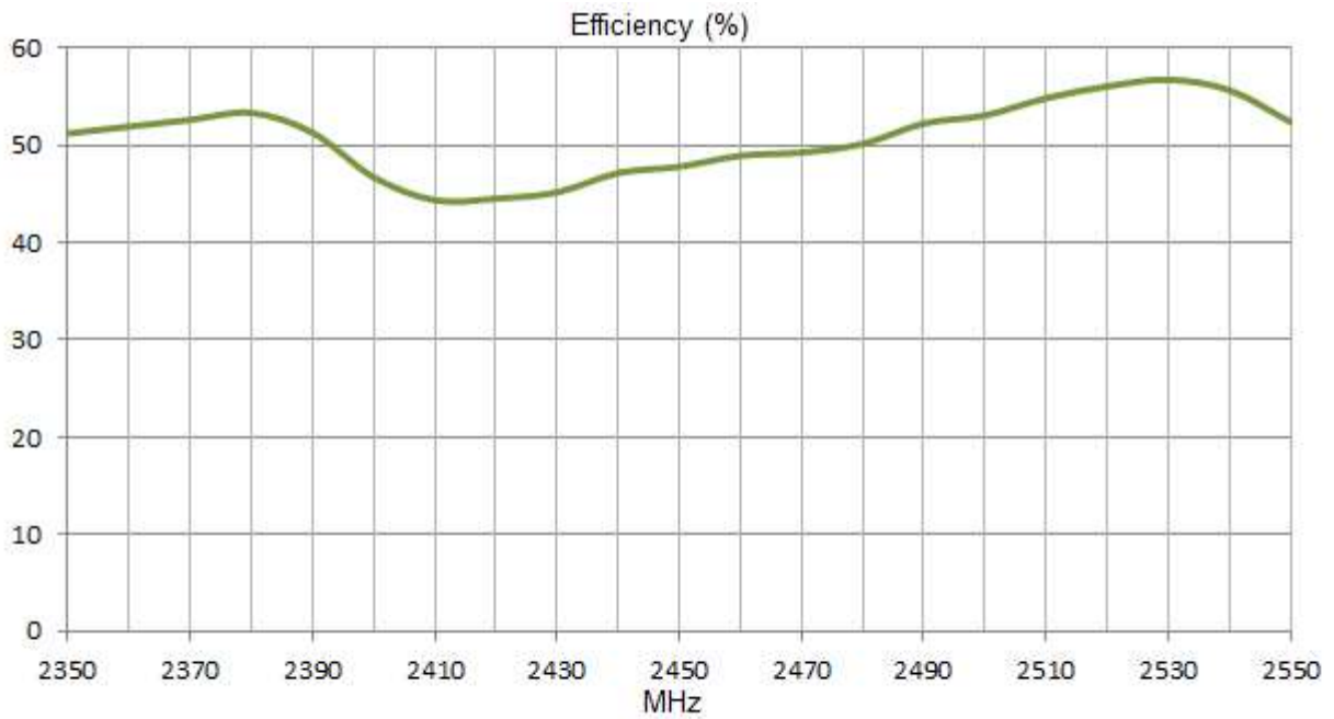
Figure 8. Efficiency of G30 Antenna at 2.4 GHz in Free Space.
