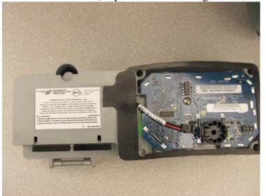
Label Location Area (on plastic frame holding radio module and battery)
