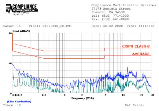
Condition: CISPR CLASS-B Test Operator:: William Zhuang Project #: : 08U11890 Company: : Silver Spring Networks Configuration:: EUT With support equipment Mode: : Normal (Hopping, Max Power) Target: : FCC Class B Voltage: : 115VAC / 60 Hz : L2: Peak ( Blue ), Average ( Green )
