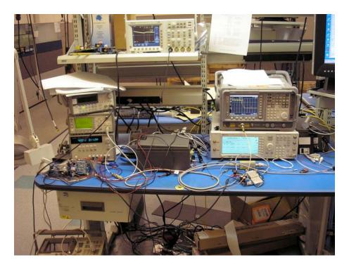
ANTENNA PORT CONDUCTED TESTS, CCS
