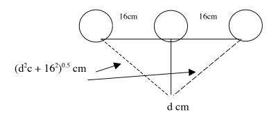
At a point located a distance d from a meter module antenna, the power density is the sum of the contributions from the center meter and the two adjacent meters. Each adjacent meters is further away, at a distance of  $(d^2c + 16^2)^{0.5}$  cm, and therefore will contribute less power density at d for the same transmitter eirp.
