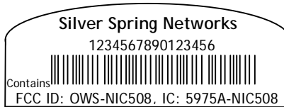
Figure 2 - Example of NIC Address Label
