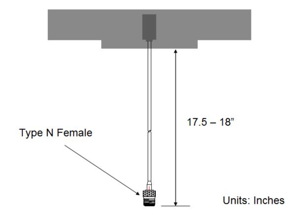
Cable: RG316/RG174 Connector: Type-N Female
