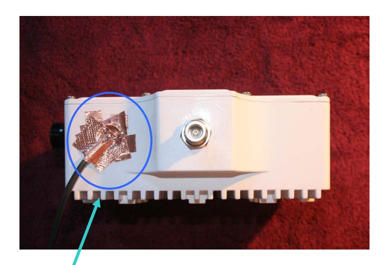
This is not present in the actual production version of the radio, this cable (USB) was installed for the certification testing only. It allows control of the radio via computer to select transmit frequency and other parameters.
