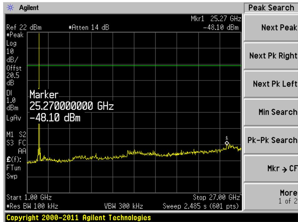
**2.4 GHz OQSK Modulation 1 Mbps data rate 5 MHz channel spacing****Low Channel**
