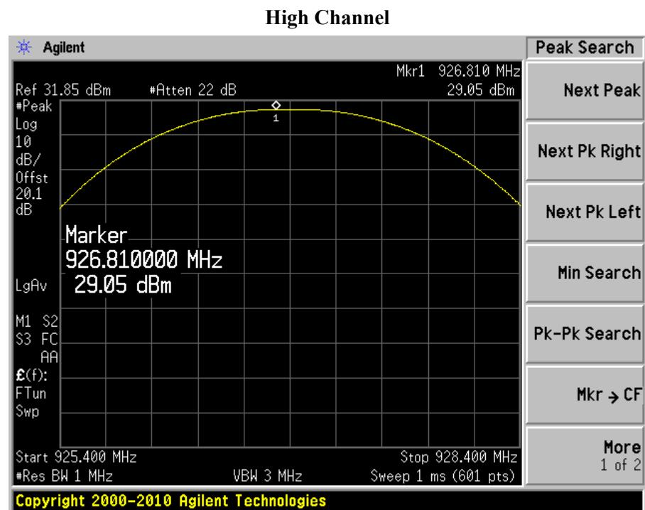
**2.4 GHz GFSK Modulation, 500 kbps data rate, 800 kHz channel spacing****Low Channel**
