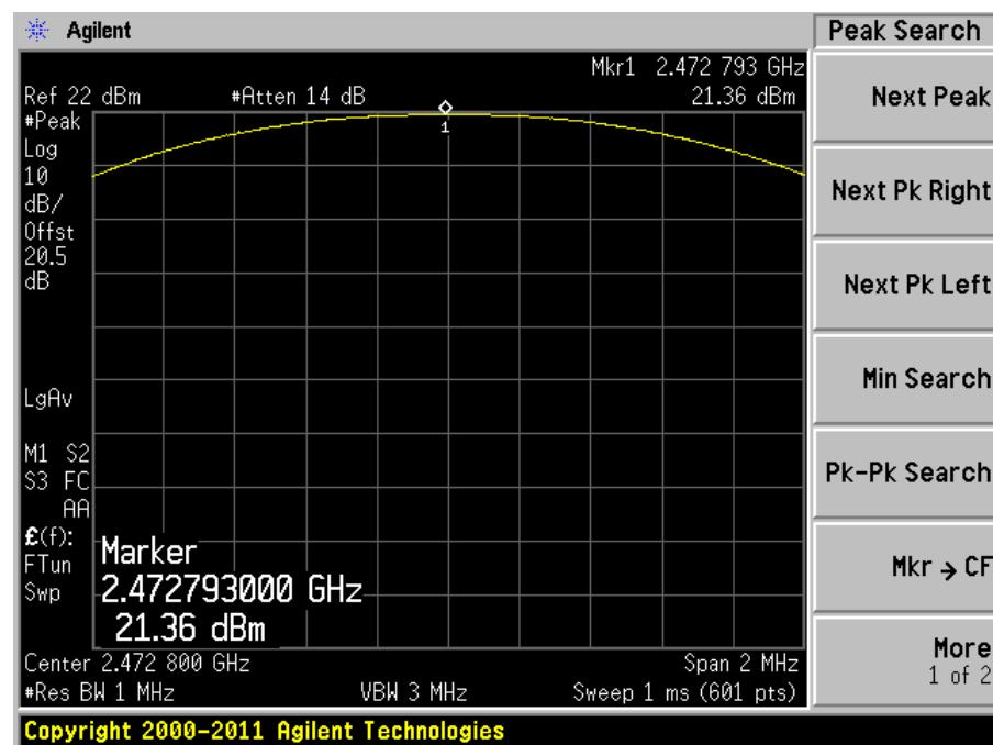
**2.4 GHz OQPSK Modulation, 1 Mbps data rate, 5 MHz channel spacing****Low Channel**
