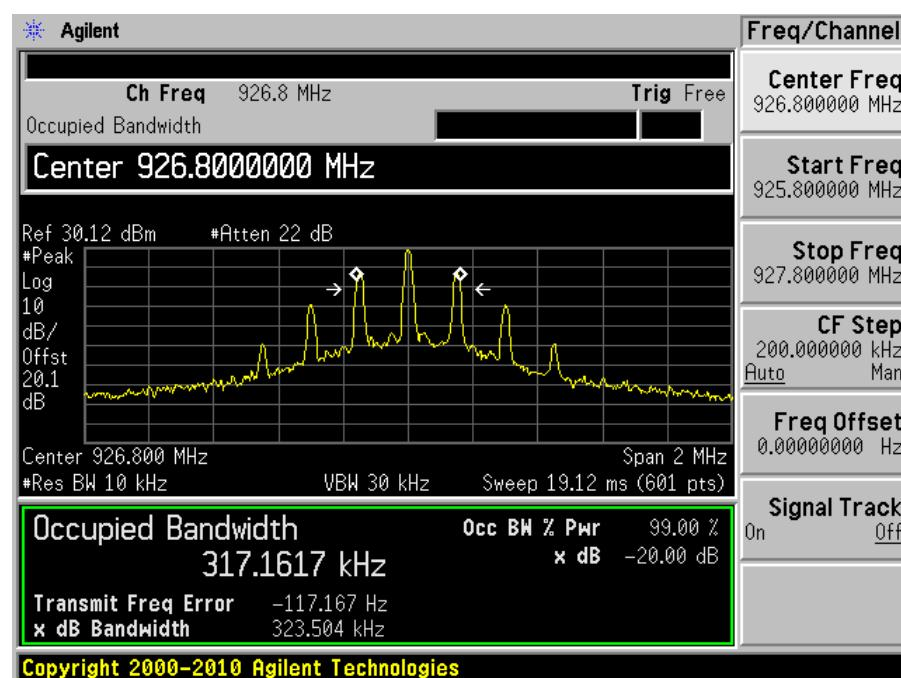
**2.4 GHz GFSK Modulation, 500 kbps data rate, 800 kHz channel spacing****Low Channel**
