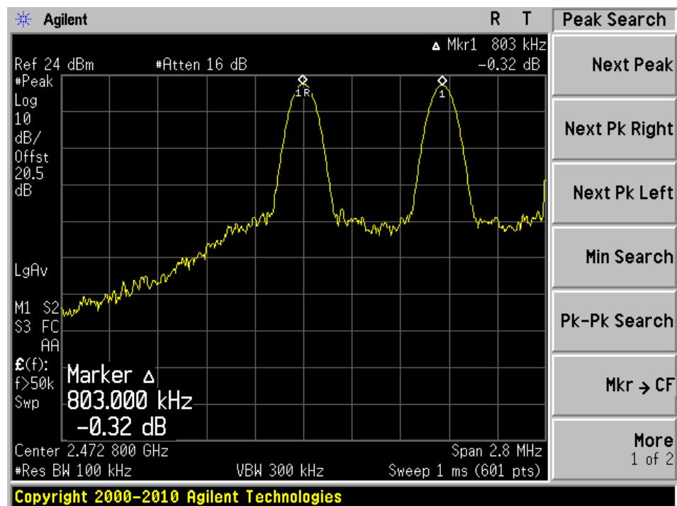
**2.4 GHz GFSK Modulation, 250 kbps data rate, 800 kHz channel spacing****Low Channel**
