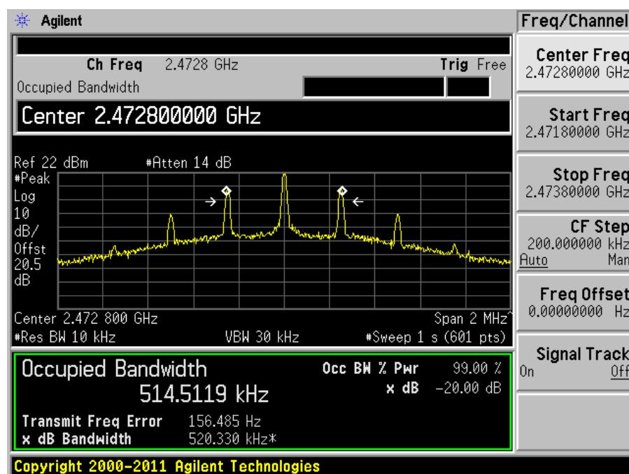
**2.4 GHz GFSK Modulation, 250 kbps data rate, 800 kHz channel spacing****Low Channel**
