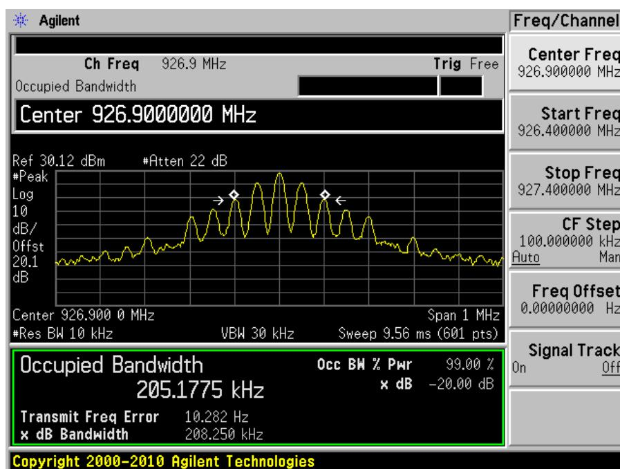
**900 MHz GFSK Modulation, 300 kbps data rate, 400 kHz channel spacing
