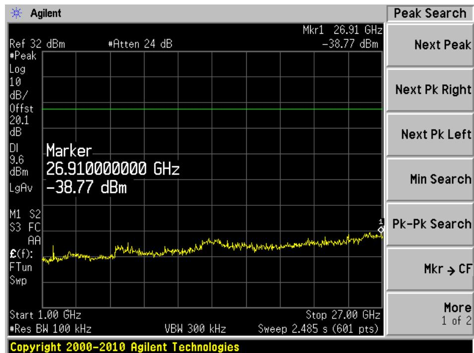
**900 MHz GFSK Modulation 300 kbps data rate 400 kHz channel spacing****Low Channel**
