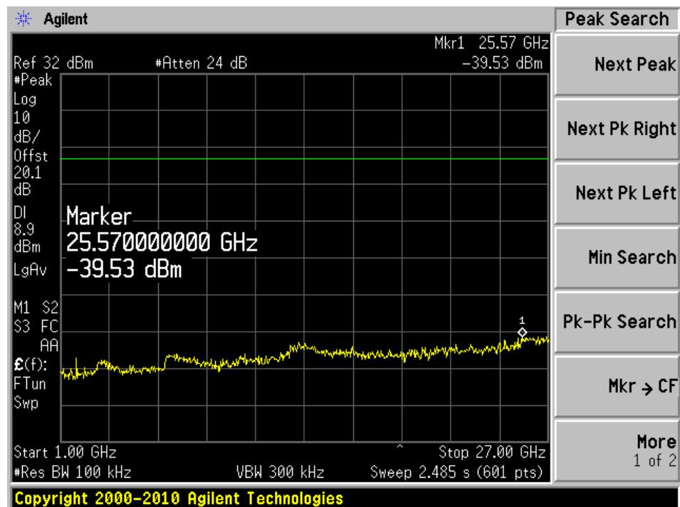
**2.4 GHz GFSK Modulation 500 kbps data rate 800 kHz channel spacing****Low Channel**
