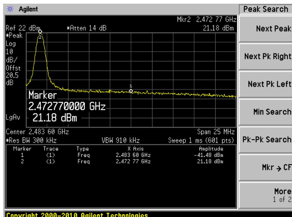
**2.4 GHz GFSK Modulation, 250 kbps data rate, 800 kHz channel spacing****Low Channel**
