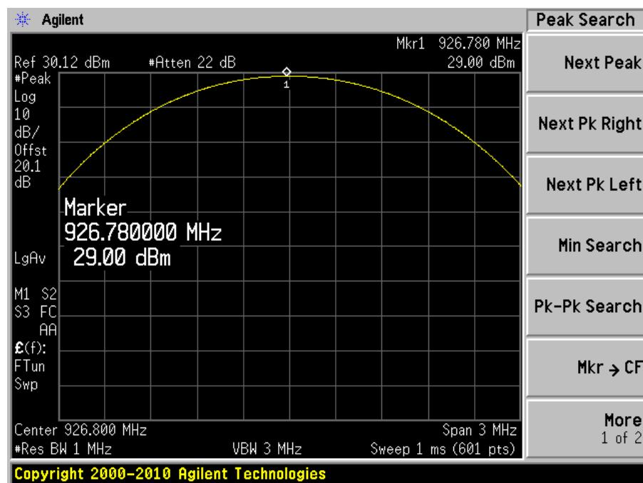
**900 MHz GFSK Modulation, 300 kbps data rate, 300 kHz channel spacing****Low Channel**
