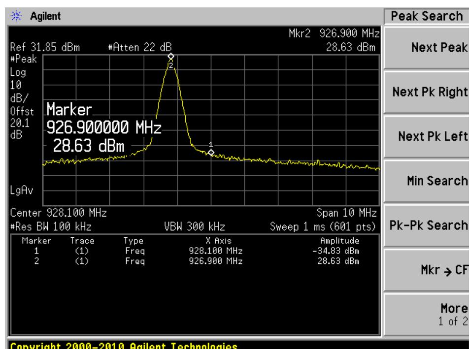
**2.4 GHz GFSK Modulation, 500 kbps data rate, 800 kHz channel spacing****Low Channel**
