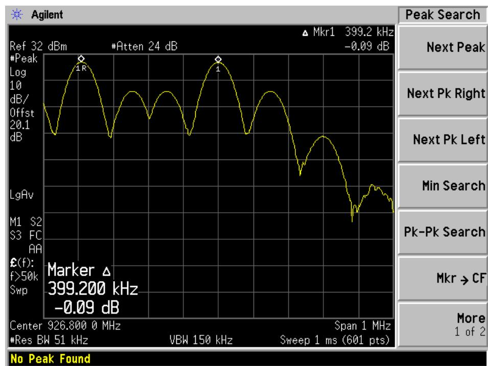
**2.4 GHz GFSK Modulation, 500 kbps data rate, 800 kHz channel spacing****Low Channel**
