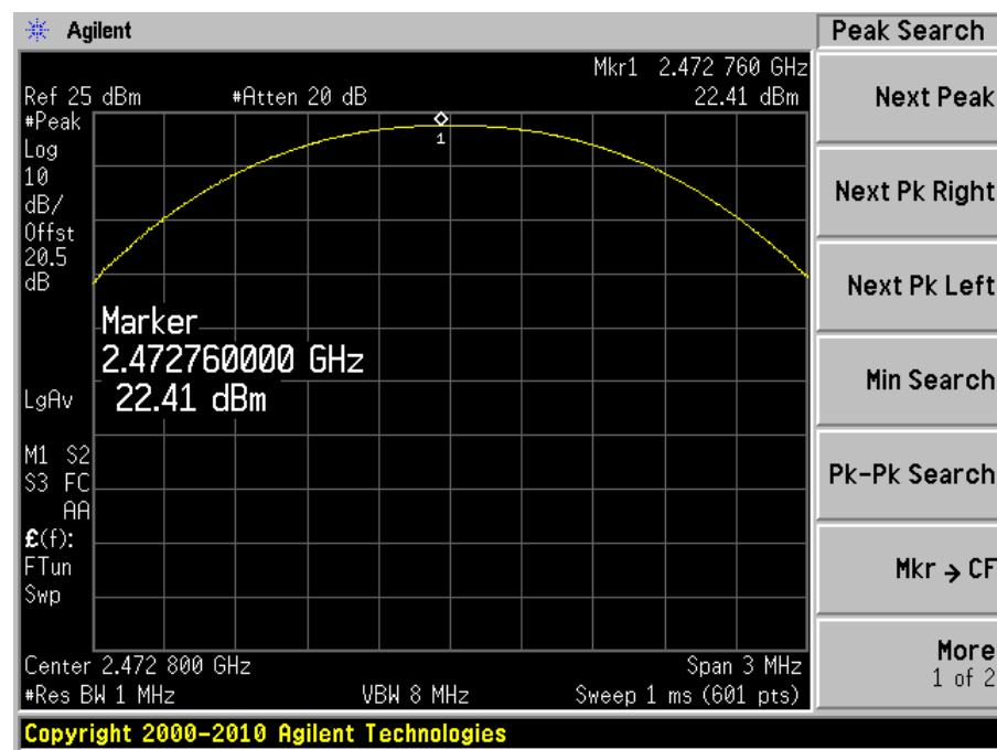
**2.4 GHz GFSK Modulation, 250 kbps data rate, 800 kHz channel spacing****Low Channel**
