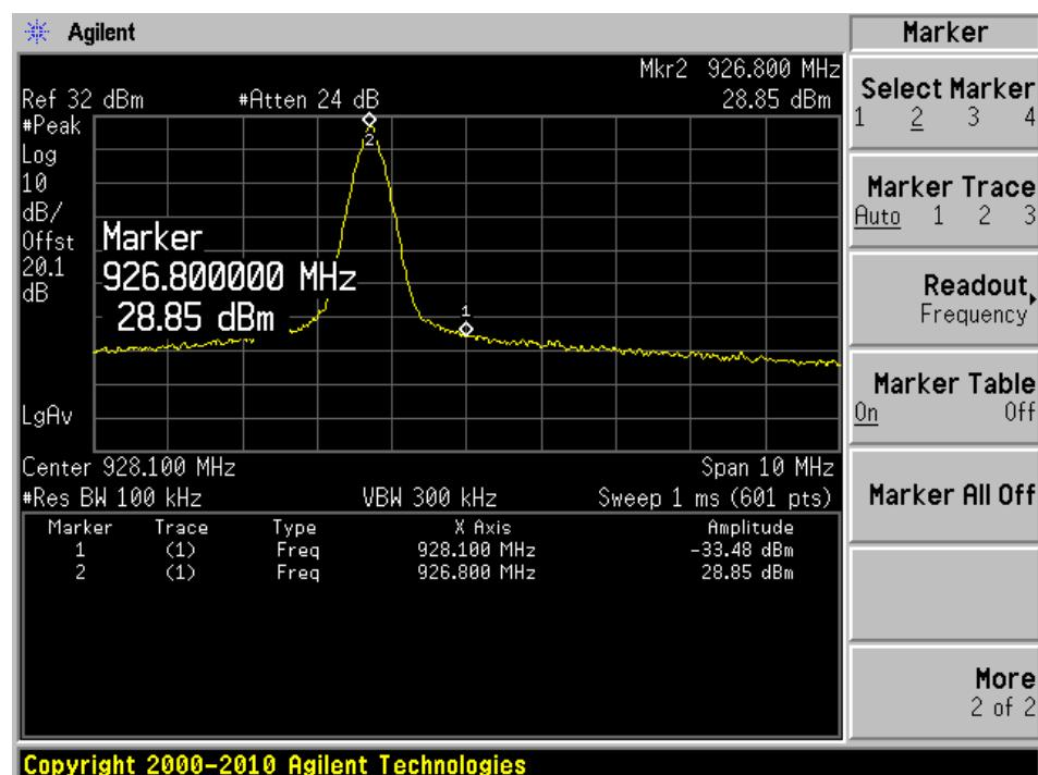
**900 MHz GFSK Modulation, 300 kbps data rate, 300 kHz channel spacing****Low Channel**
