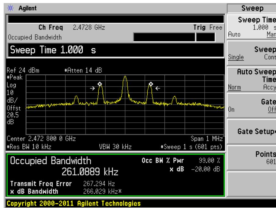
**2.4 GHz OQPSK Modulation, 1 Mbps data rate, 5 MHz channel spacing****Low Channel**
