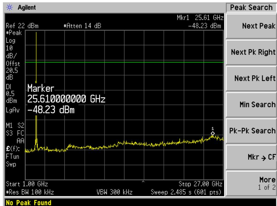
**2.4 GHz GFSK Modulation 250 kbps data rate 800 kHz channel spacing****Low Channel**
