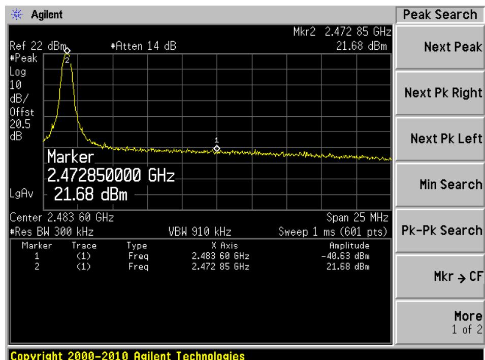
**2.4 GHz OQPSK Modulation, 1 Mbps data rate, 5 MHz channel spacing****Low Channel**
