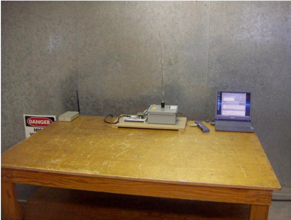
AC Line Conducted test set-up
