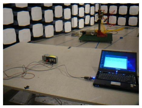
NOTE: Laptop and serial cable were removed after EUT parameters were set and the EUT was transmitting continuously at the desired channel and power.
