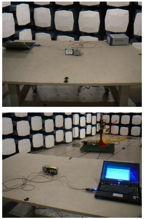
NOTE: Laptop and serial cable were removed after EUT parameters were set and the EUT was transmitting continuously at the desired channel and power.
