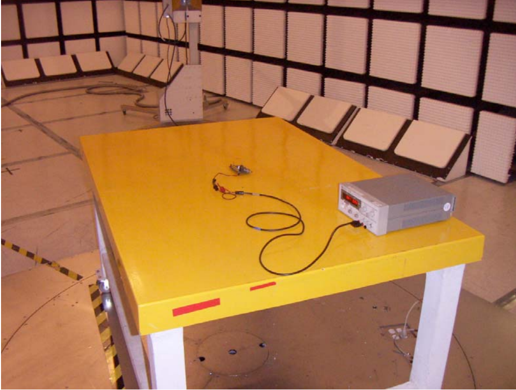
Radiated Emissions Test Setup, Worst-case Orientation (“X” orientation) – power supply
