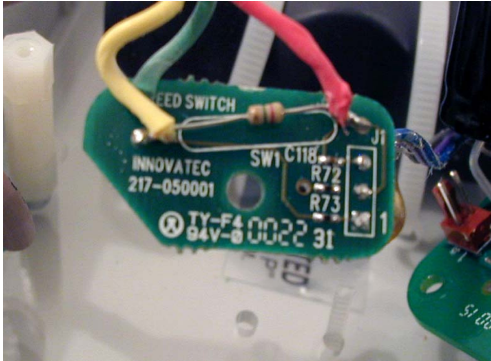
Figure 7 Component Side View of Reed Switch Board
