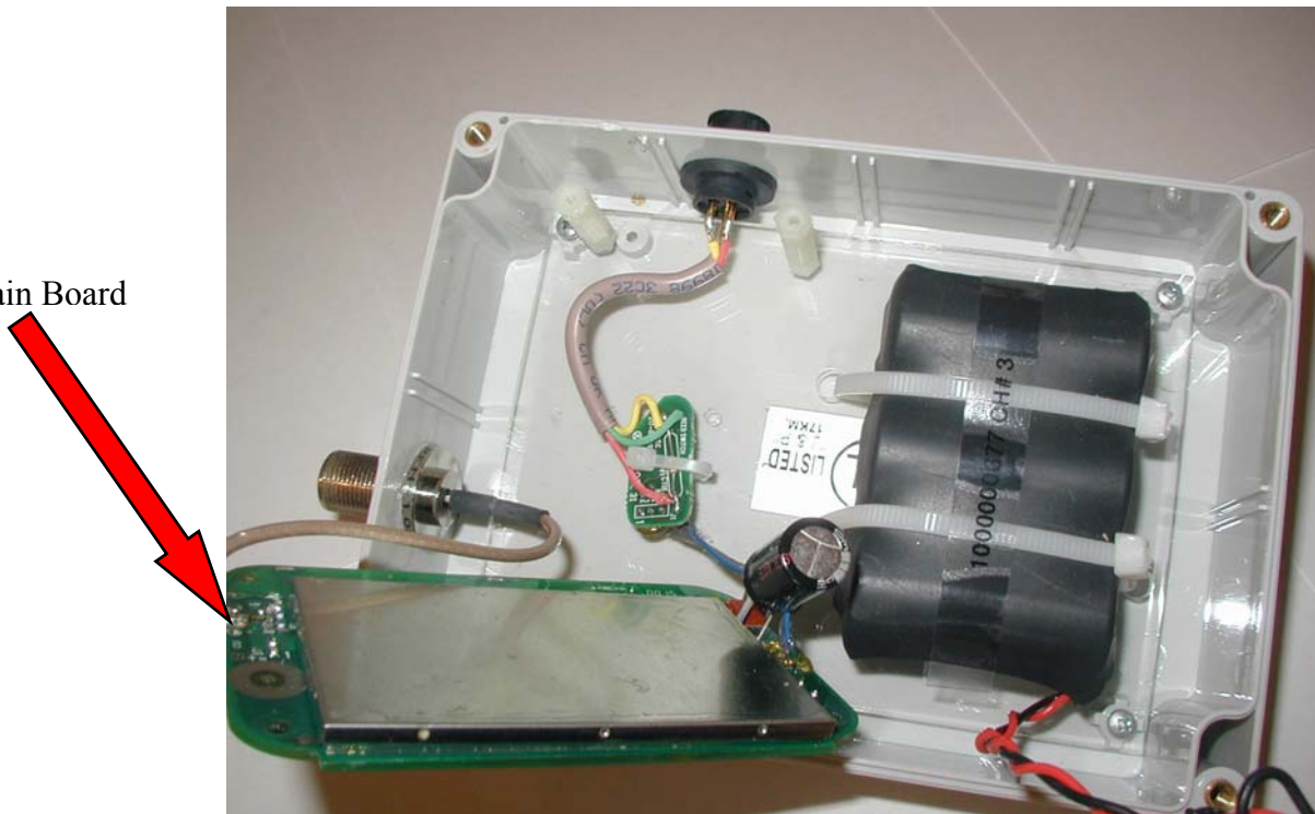
Figure 4 Overhead View of EUT with Main Board Removed
