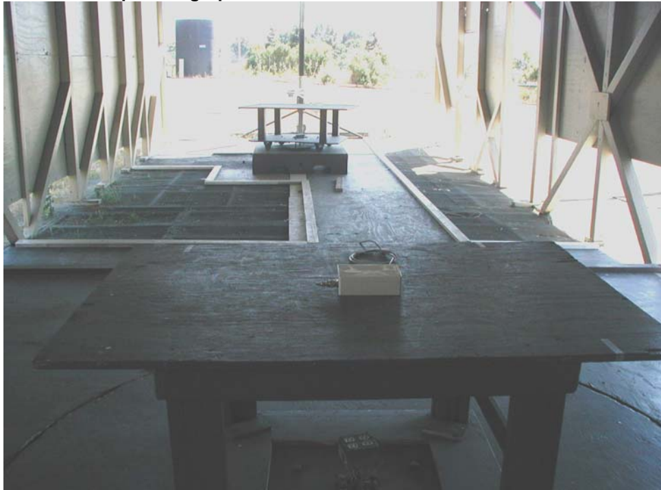
Figure 1: Spurious Emissions Test Setup at 10 meters (30MHz to 1000MHz)
