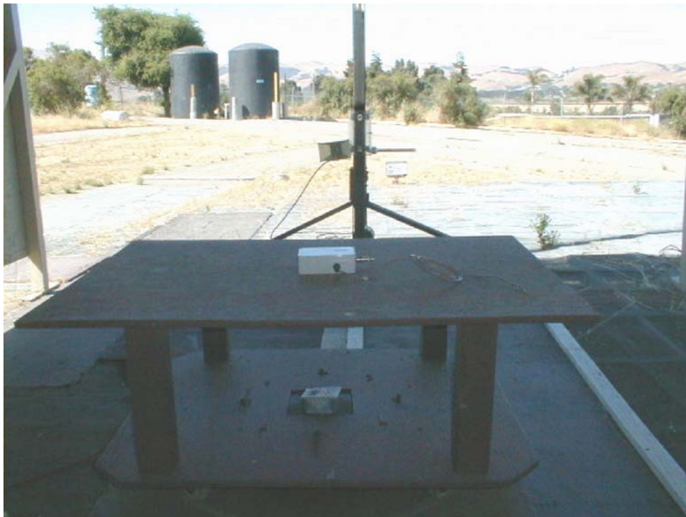
Figure 2 Radiated Emissions Test Setup at 3 meters (above 1GHz)
