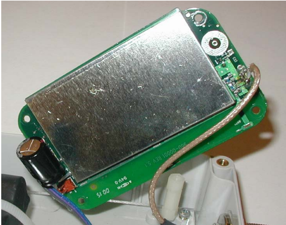
Figure 5 Main-Board Antenna Side View with Shield Cover
