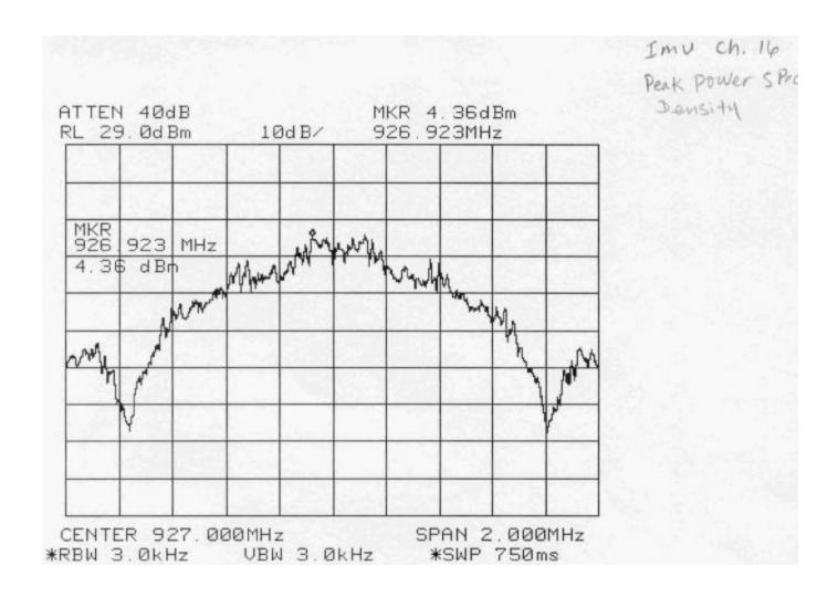
The conductive peak power density did not exceed 8 dBm as required per section 15.247(d).
