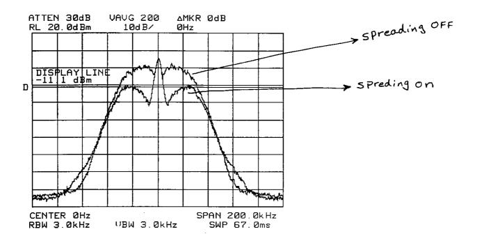
\* measured Processing Gain > 11 dB
