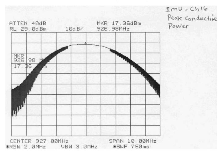
The maximum conductive peak power did not exceed 1 watt as required per section 15.247.
