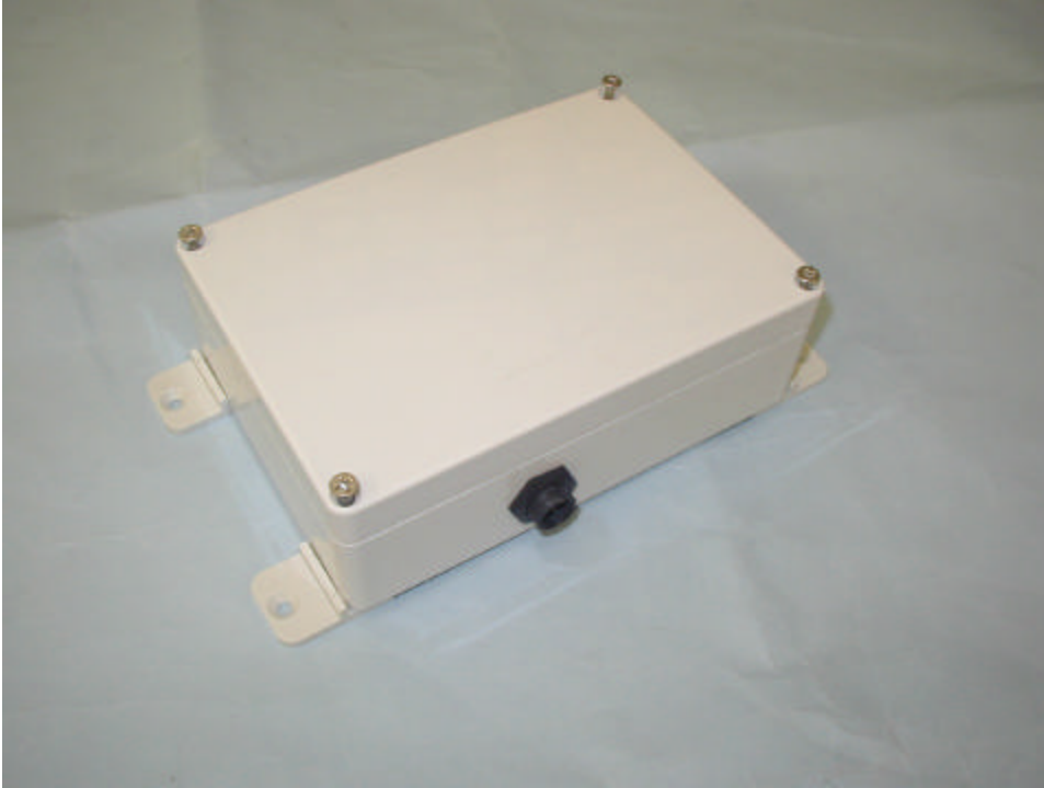
Top View of C & I Gas Meter Interface
