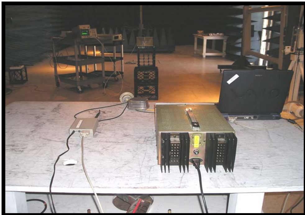
Figure 4: Radiated Emissions Test Setup (Above 1 GHz) Rear View
