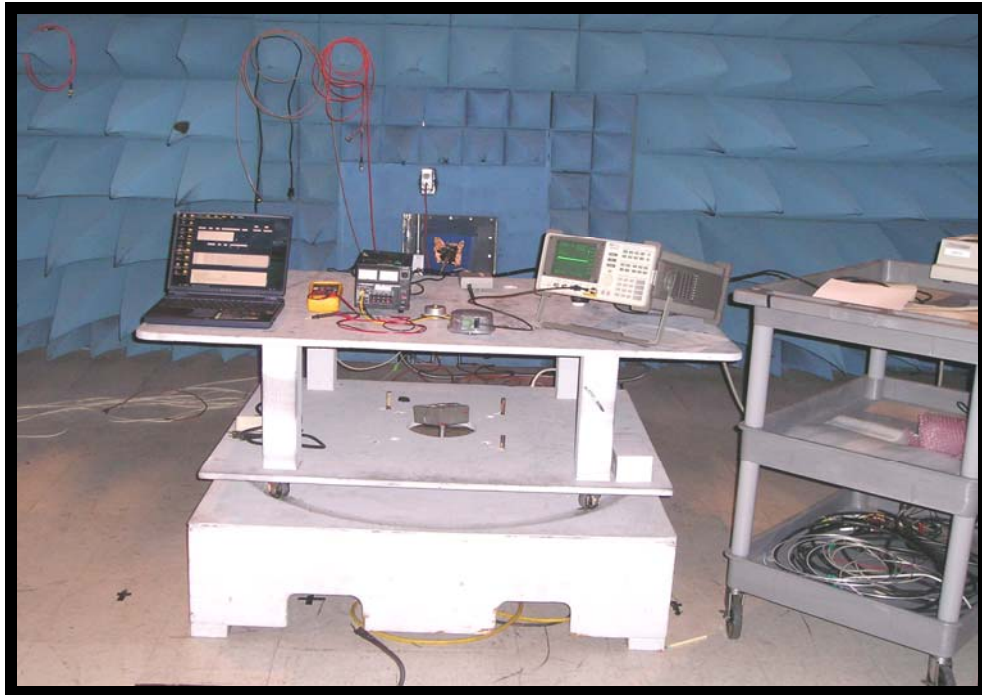
Figure 5 Test Set Up Photos – RF Conducted (Front View)
