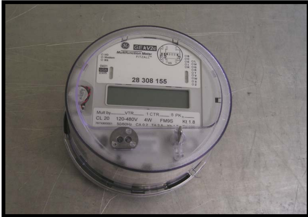
Figure 3: kV2C with internal antenna (Top View)
