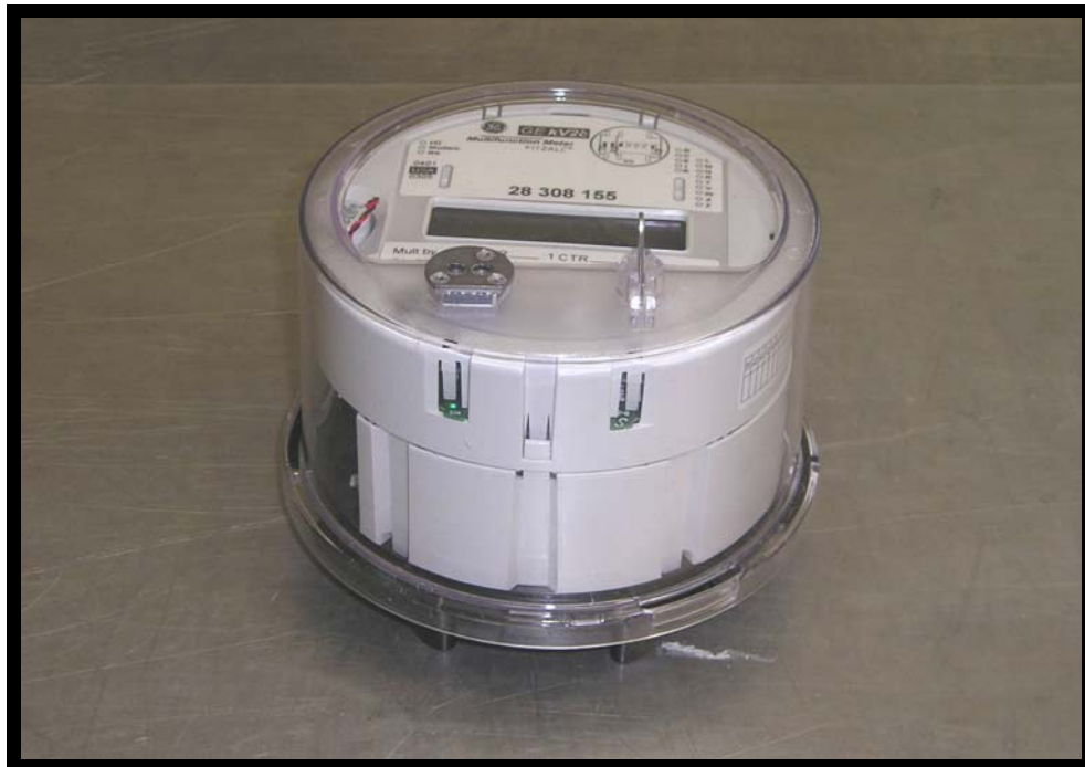
Figure 4: kV2C with internal antenna (Front View)
