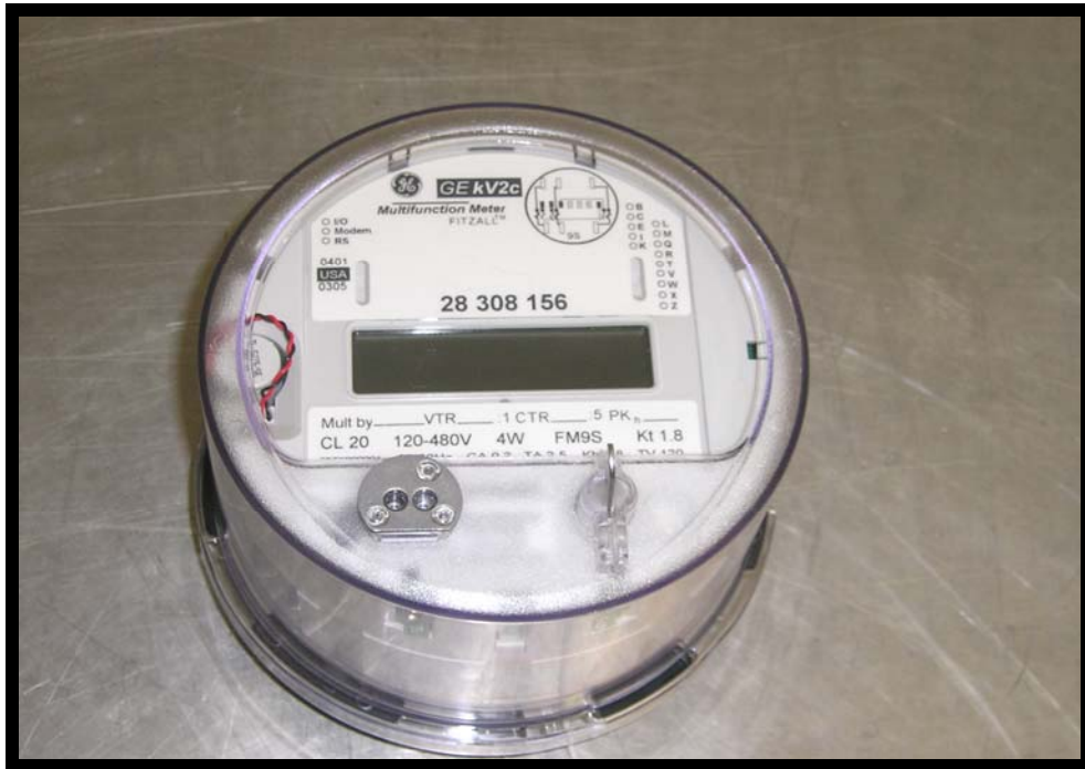
Figure 1: kV2C with external antenna (Top View)
