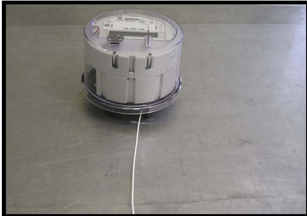
Figure 2: kV2C with external antenna (Front View)
