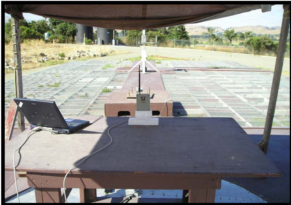
Figure 32: Spurious Emissions Rear View (Below 1 GHz)
