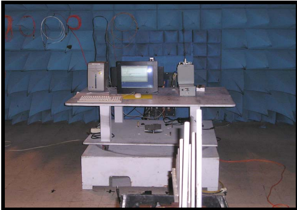
Figure 7: Power Spectral Density Test Setup (Front view)
