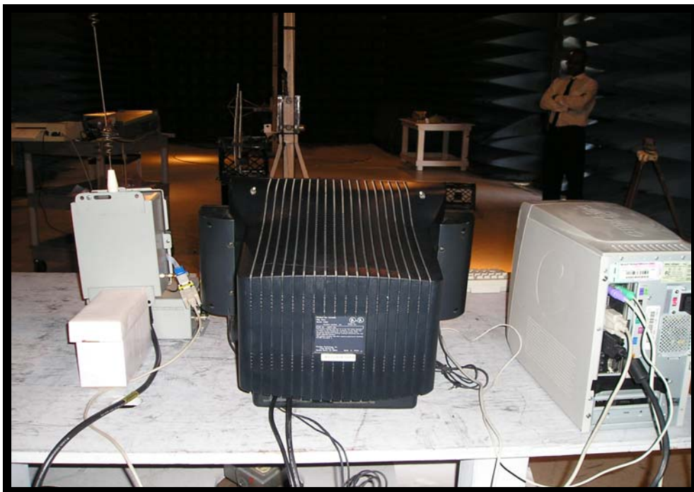
Figure 16: Power Spectral density Test Setup (Rear View)
