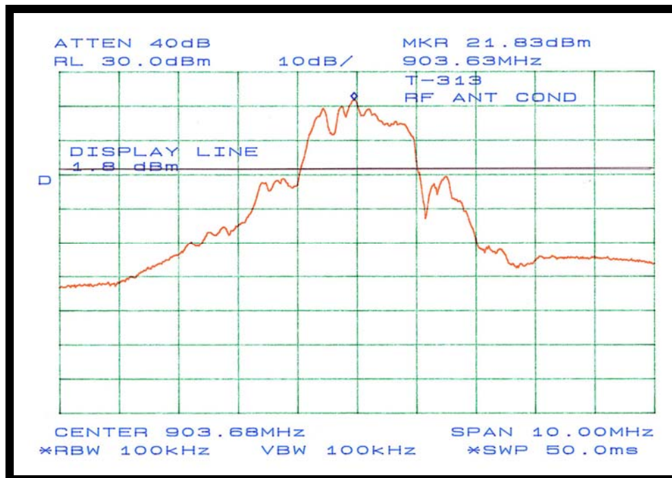
Figure 22: Plot of 100 kHz Bandwidth Out-of-Band Measurement (In-Band-Peak)
