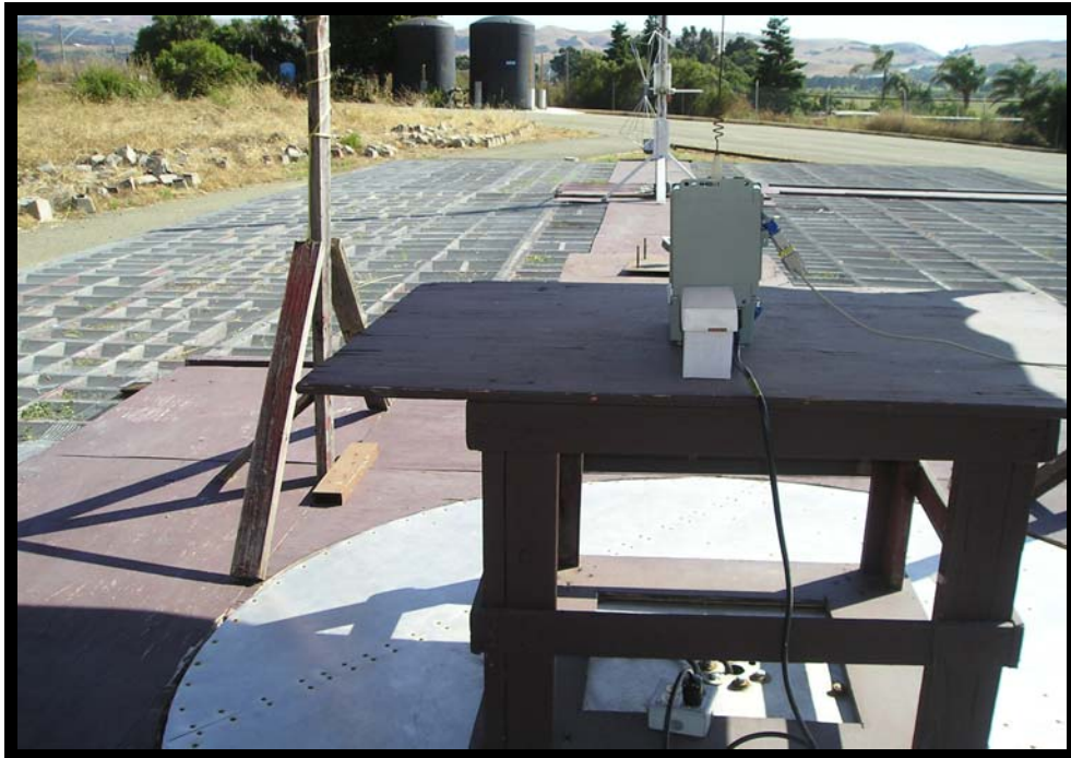
Figure 2 Radiated Emissions Test Setup (Below 1 GHz) Rear View
