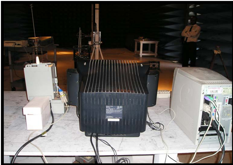
Figure 8: Power Spectral density Test Setup (Rear View)
