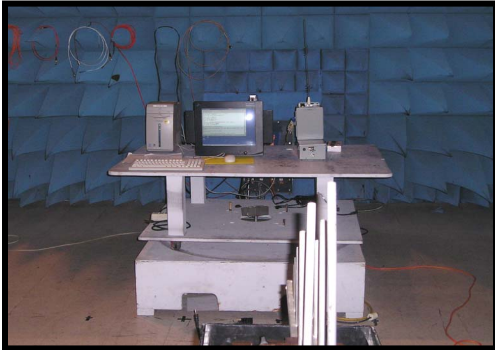
Figure 15: Power Spectral Density Test Setup (Front view)
