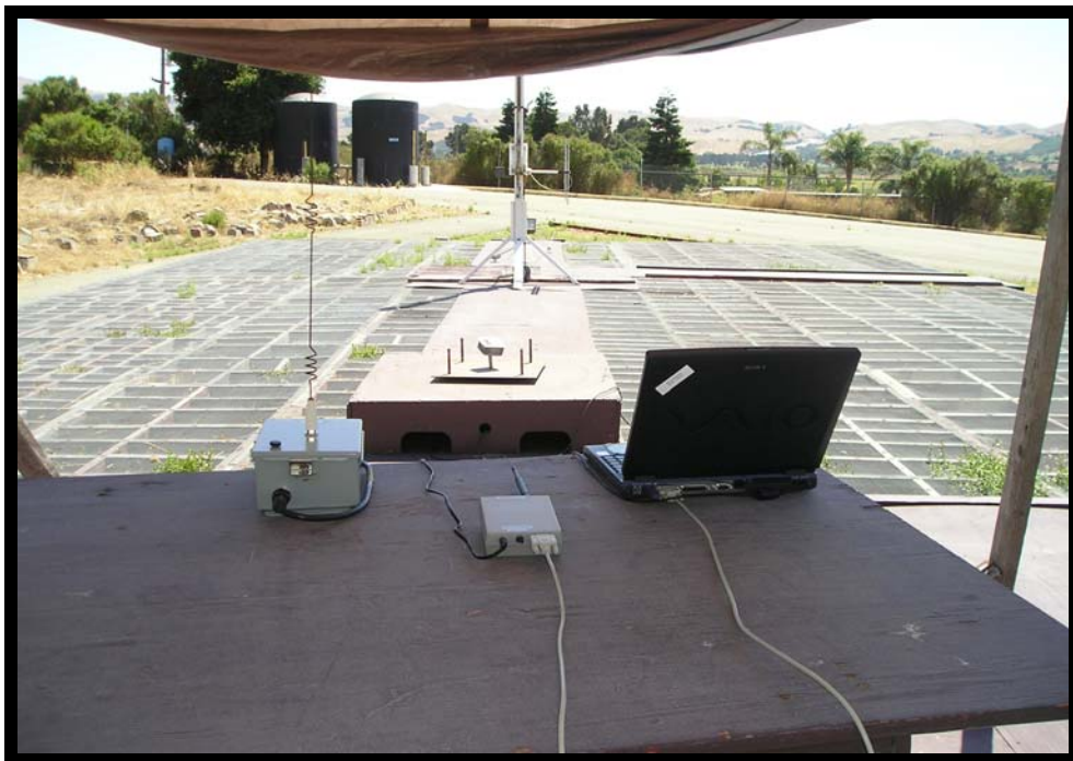
Figure 10 Spurious Emissions Test Setup (Below 1 GHz) Rear View
