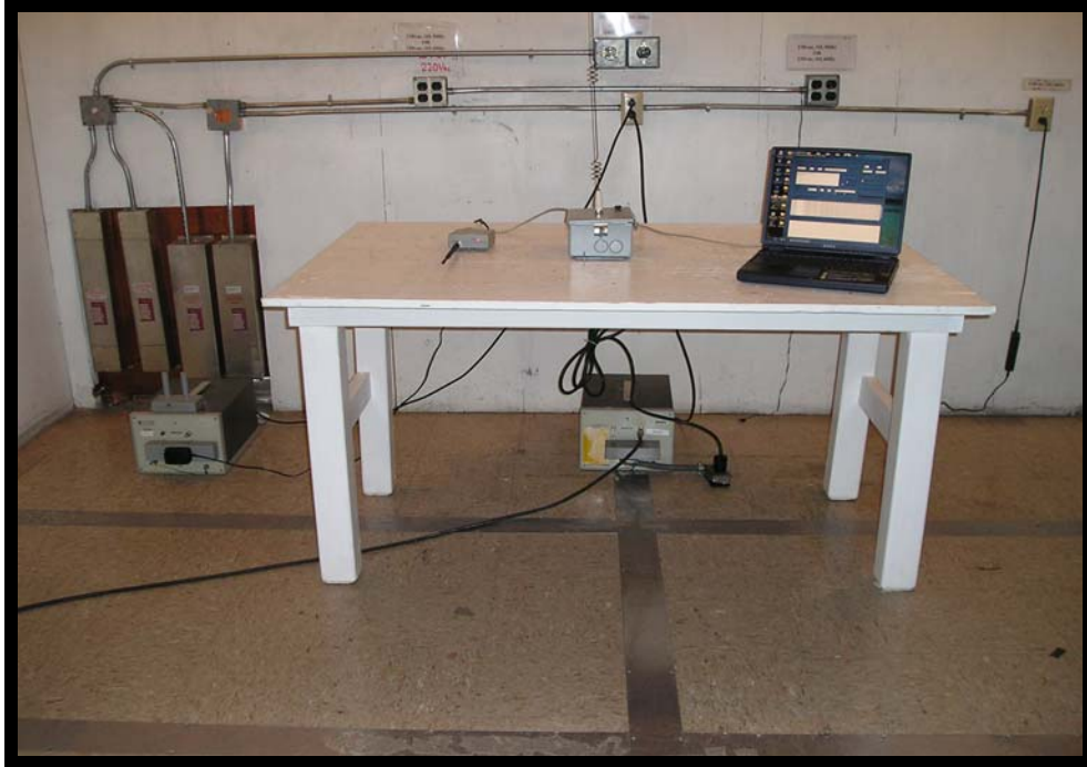
Figure 13: Power Line Conducted Maximized Emissions Test Setup (Front View)
