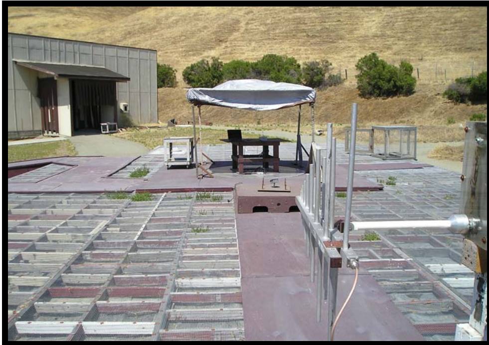
Figure 9: Spurious Emissions Test Setup (Below 1 GHz) Front View
