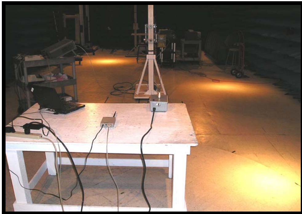
Figure 12: Spurious Emissions Test Setup (Above 1 GHz) Rear View.
