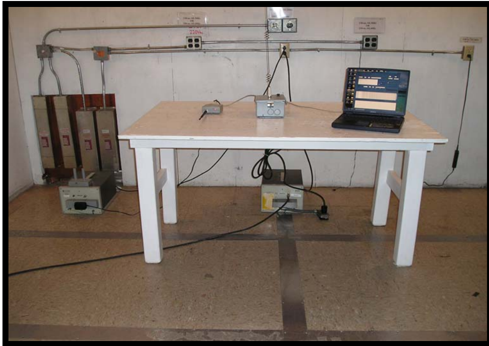
Figure 36: Power Line Conducted Maximized Emissions Test Setup (Front View)
