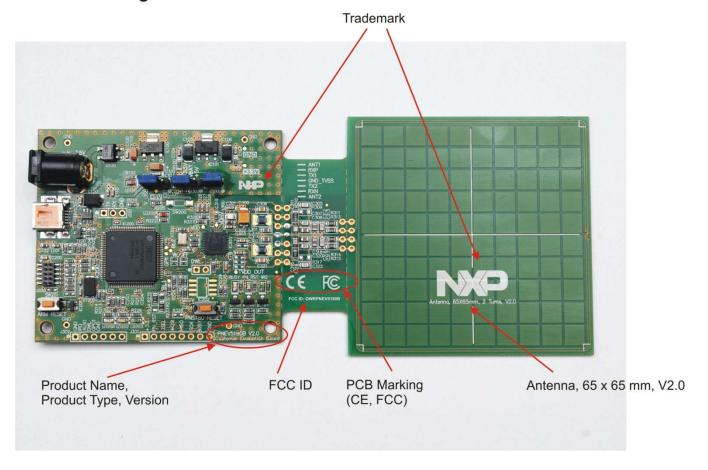
PCB Marking and Label for Customer Evaluation Board PNEV5180B V2.0 with FCC ID: OWRPNEV5180B
