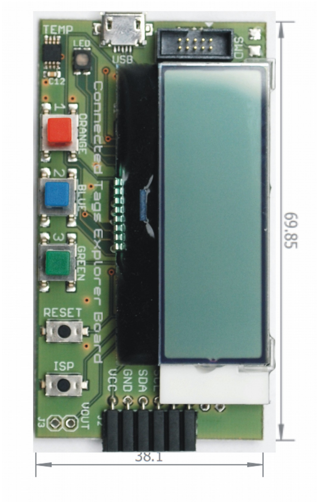
Figure 7: Connected Tags Explorer Board OM5569, Rev. 2.0: dimensions and equipped pcb with connectors.
