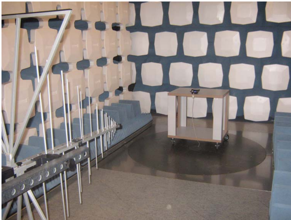
Figure 3: Radiated emission test – 30MHz to 1GHz
