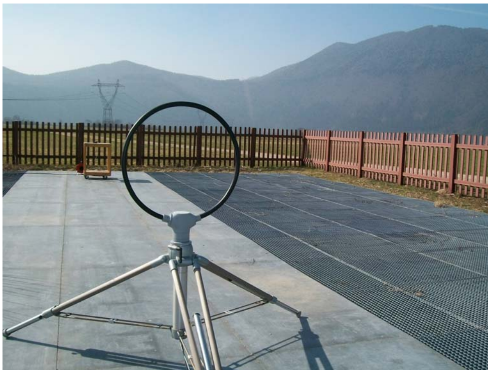
Figure 4: Radiated emission test – OATS measurements
