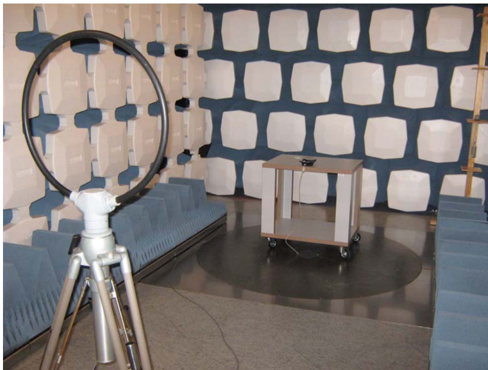
Figure 2: Radiated emission test – 9 kHz to 30 MHz
