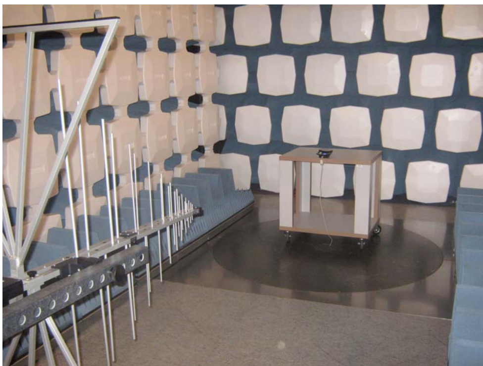
Figure 3: Radiated emission test – 30MHz to 1GHz
