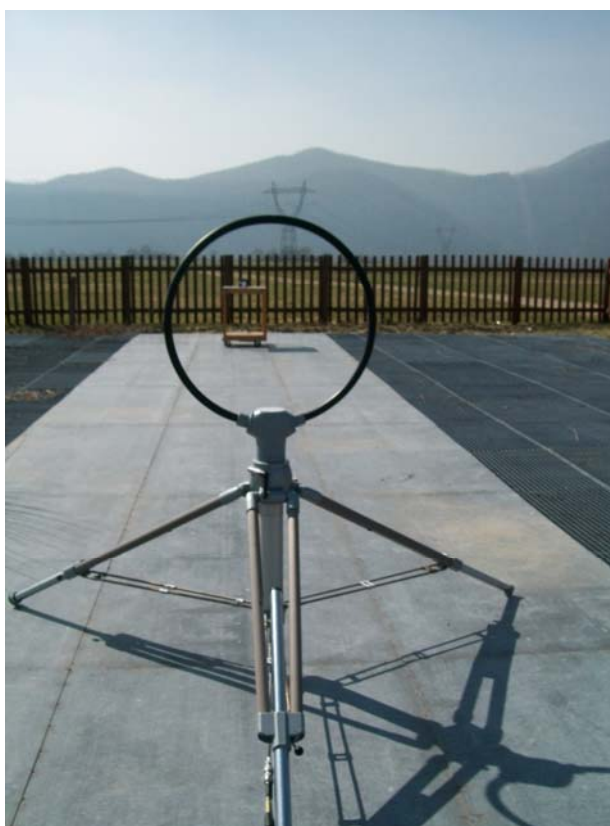
Figure 4: Radiated emission test – OATS measurements
