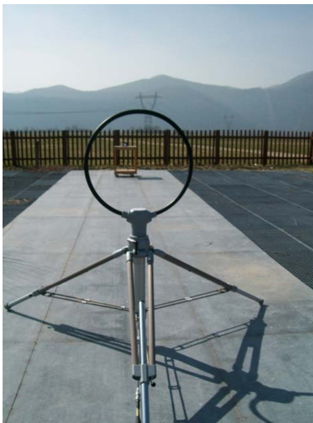
Figure 4: Radiated emission test – OATS measurements
