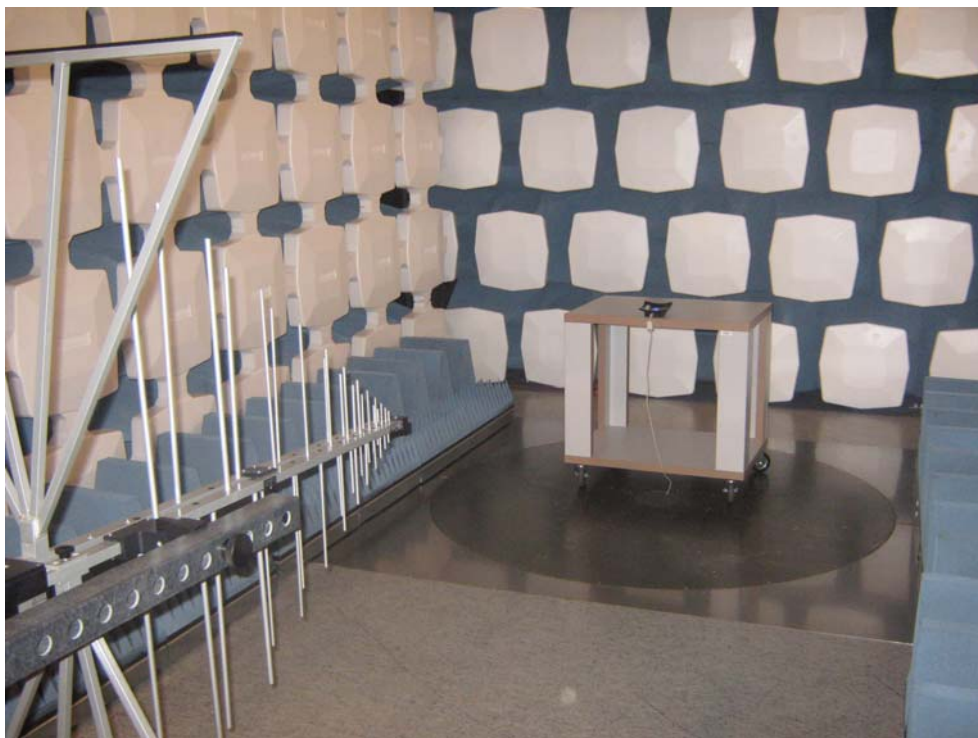
Figure 3: Radiated emission test – 30MHz to 1GHz
