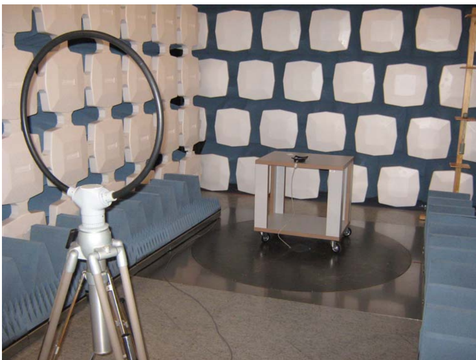
Figure 2: Radiated emission test – 1MHz to 30MHz
