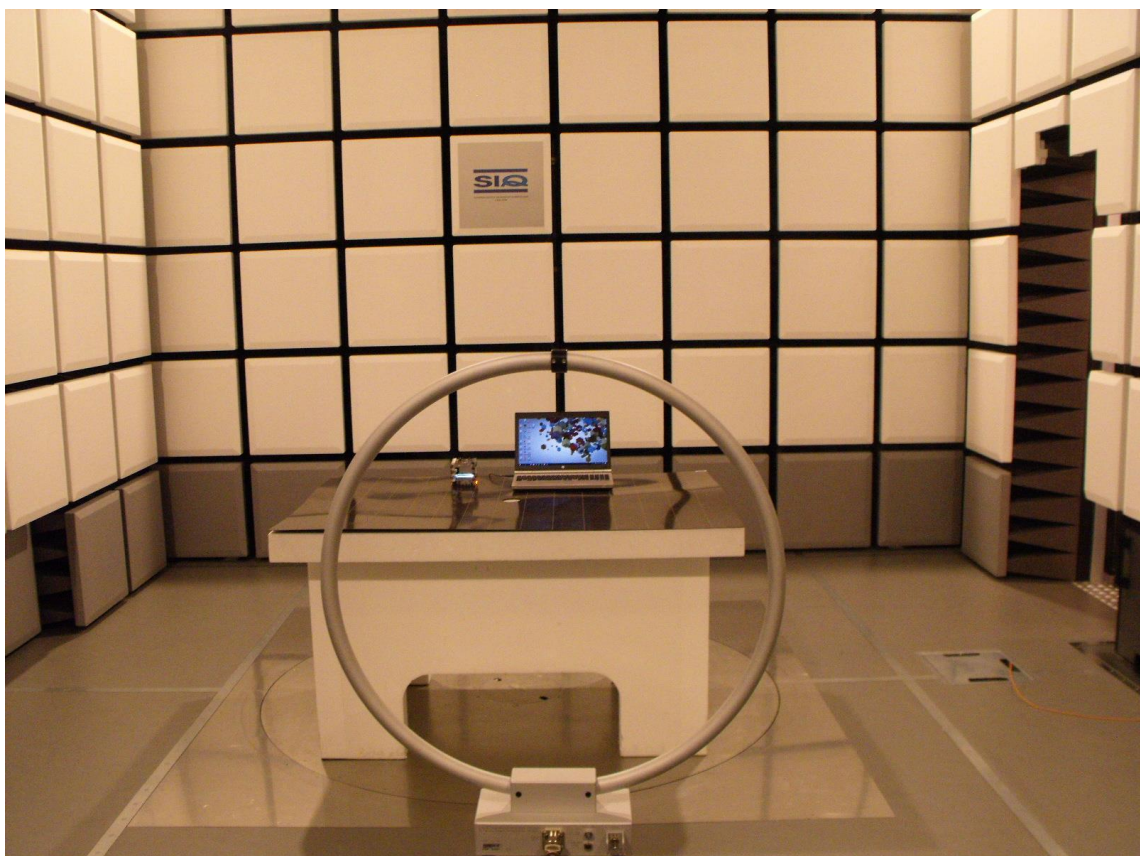
Figure 2: Radiated emission test from 9 kHz to 30 MHz
