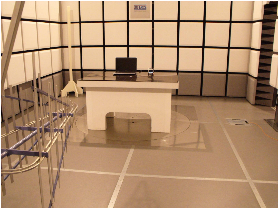
Figure 6: Radiated emission test from 200 MHz to 1 GHz
