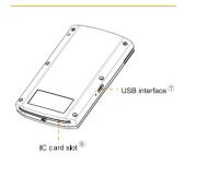
Dual color charging indicator for operation status, which may change in response to different application configuration Mag-stripe card swiping position, swiping slot 3 bidirectional Display transaction and operation tips Display screen 4 Input amount and code, confirm and Keypad <sup>⑤</sup> cancel transaction etc., long press the cancel key to turn on or off Contactless IC card read-write induction Can be charged by connecting to PC or Contact IC card inserting position
