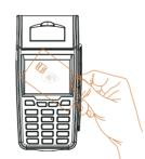
When the screen display "Please sign", please guide customer to sign in the blank area by the customized stylus; after that, pressing the enter key means complete this operation, while pressing the cancel key will exit this operation.
