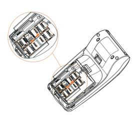
3 Don't attach any item, which will increase the card thickness, like sticker and tag, to the SIM/SAM card, lest the failure of installment and disassembly.
