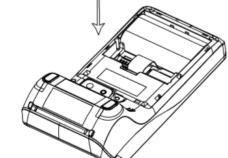
(2) Insert the plug side of the battery into the battery socket; 3) Put the battery into the battery container; (4)Close the battery cover.
