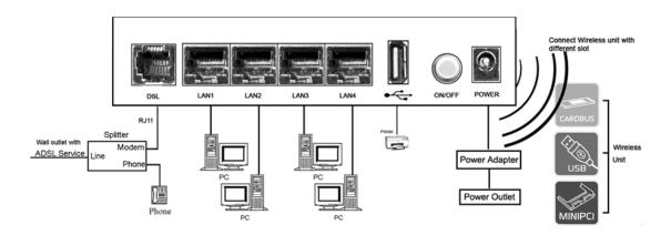
Notes: Without the splitter and certain situation, transient noise from telephone can interfere with the operation of the Router, and the Router may introduce noise to the telephone line. To prevent this from happening, a small external splitter must be connected to each telephone.
