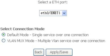
3. Select a ETH port as you will. You can select ENET1, ENET2, ENET3 or ENET4 port as the WAN interface and MSC mode as connection mode.
