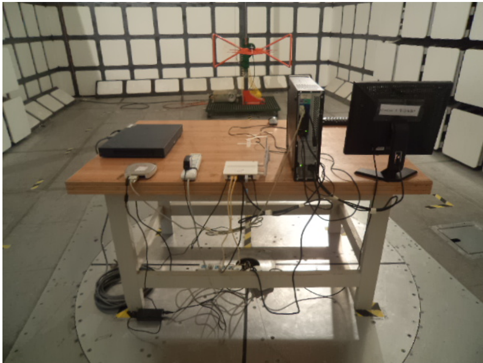
Spurious Radiated Emissions – Rear View (30 MHz - 1 GHz)
