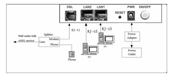
Notes: Without the splitter and certain situation, transient noise from telephone can interfere with the operation of the Router, and the Router may introduce noise to the telephone line. To prevent this from happening, a small external splitter must be connected to each telephone.
