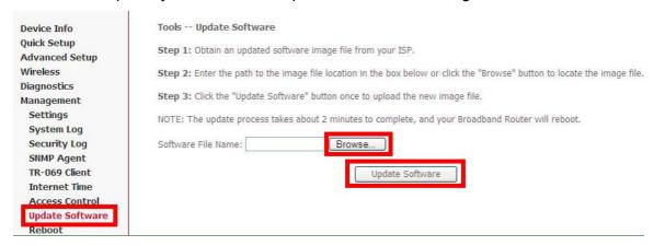
Note: Be sure that the firmware you want to update is the same product model as yours. Do not turn off the power when the updating is not finished! When it finished, you can't turn back to the default version unless you have the previous firmware!
