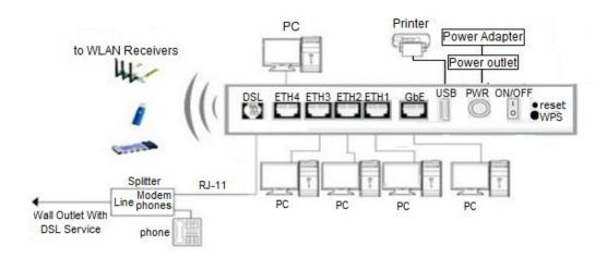
Notes: Without the splitter and certain situation, transient noise from telephone can interfere with the operation of the Router, and the Router may introduce noise to the telephone line. To prevent this from happening, a small external splitter must be connected to each telephone.
