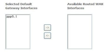
8. Get DNS server information from the selected WAN interface or enter static DNS server IP addresses. If only a single PVC with IPoA or static MER protocol is configured, you must enter static DNS server IP addresses.
