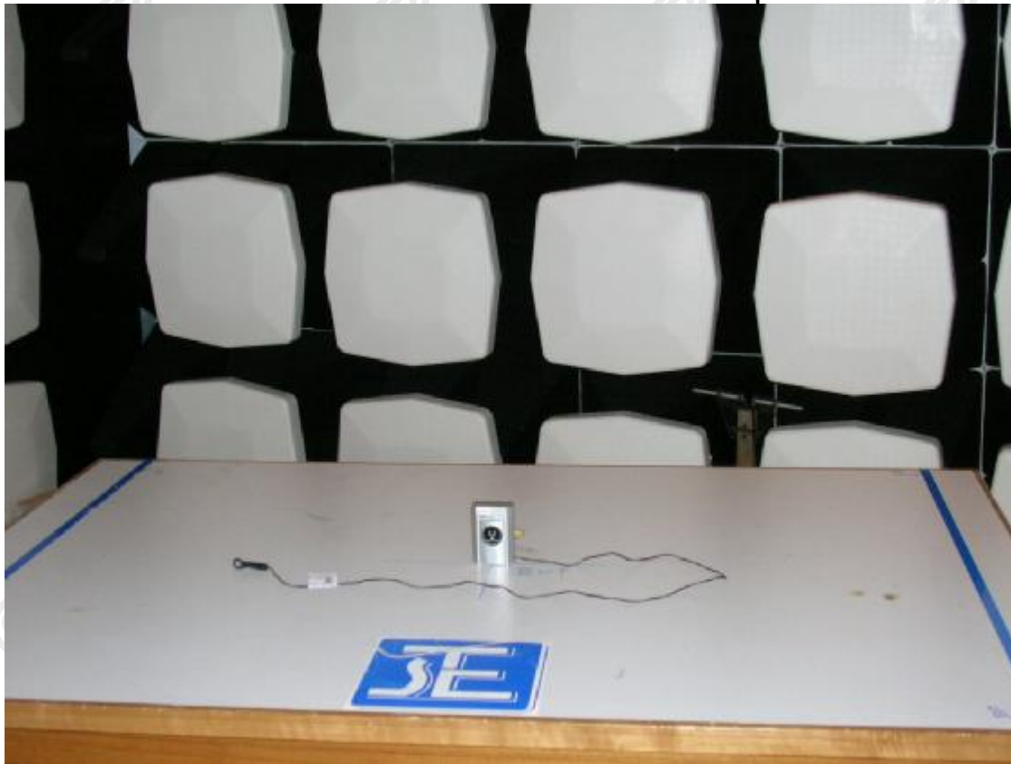
Measurement of Radiated Emission Test Set Up
