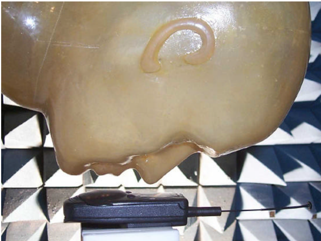
Figure 8. Diagram showing typical alignment of radio held to face.
