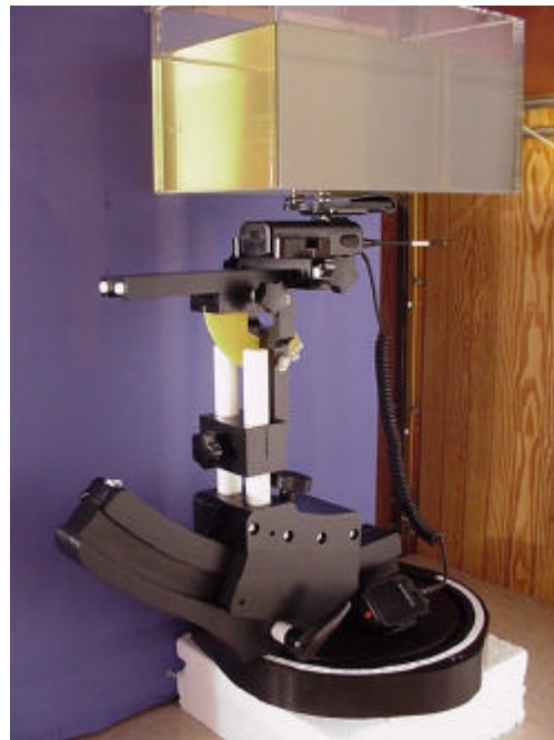
Body SAR Test Setup with small planar phantom EUT with leather belt-loop and Swivel Clip
