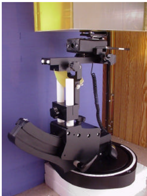
Body SAR Test Setup with small planar phantom EUT with leather belt-loop and leather case
