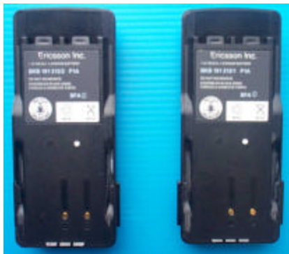
TYPES OF BATTERIES "Thick" BKB-191-212/2-P1A (left) "Thin" BKB-191-212/1-P1A (right)
