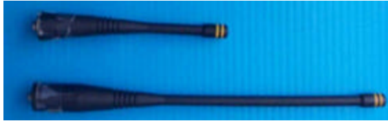
TYPES OF ANTENNAS: Helical \lambda/4 antenna S/N 11445 (top) Helical \lambda/2 antenna (bottom)
