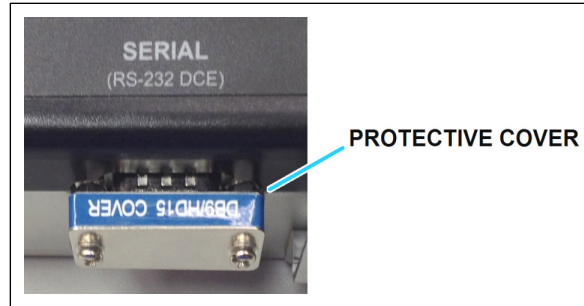
Figure 6-2: Serial Port Protective Cover for Division 2 Non-Incendive Applications
