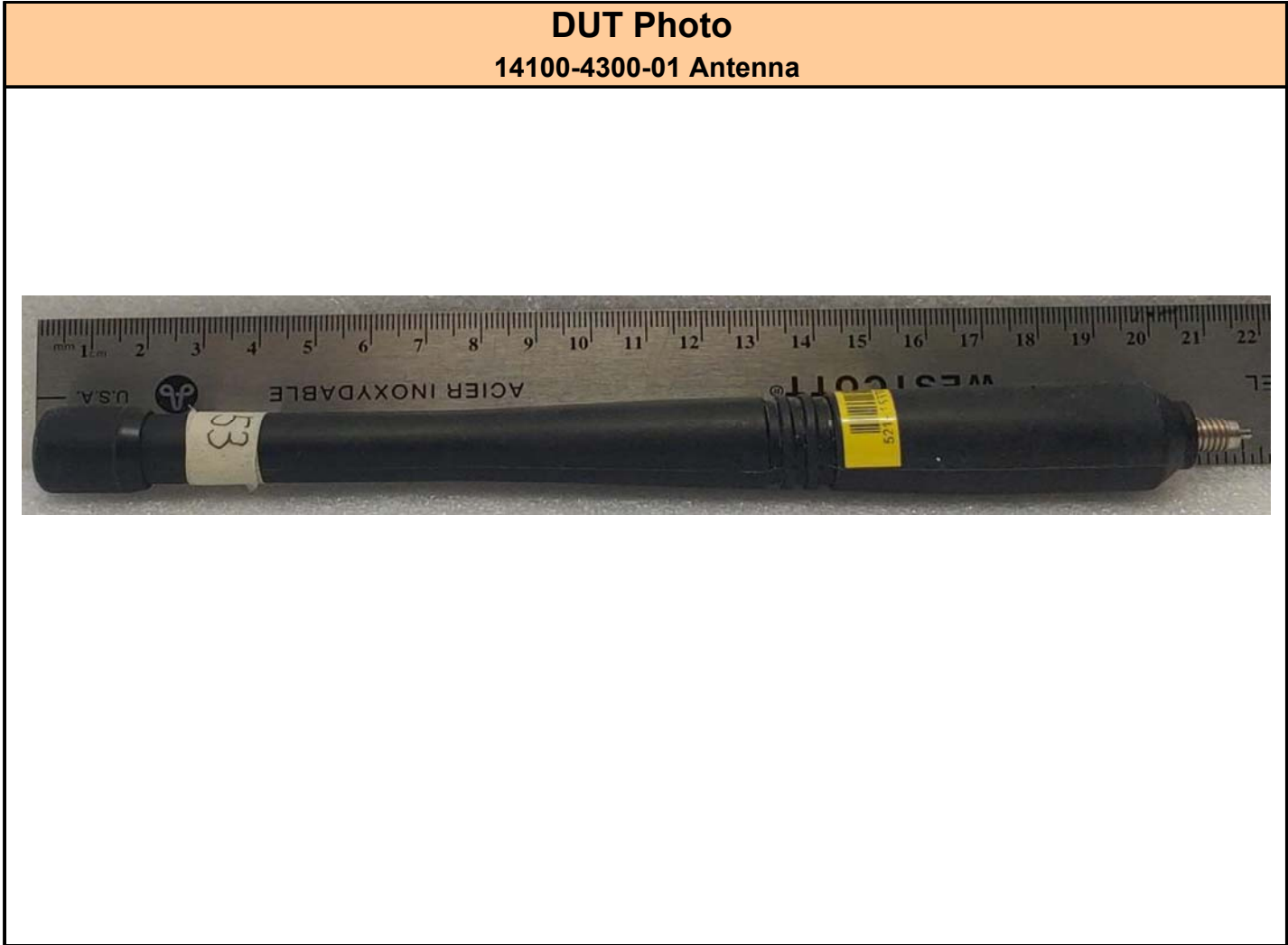
Figure D.5 – Antenna
